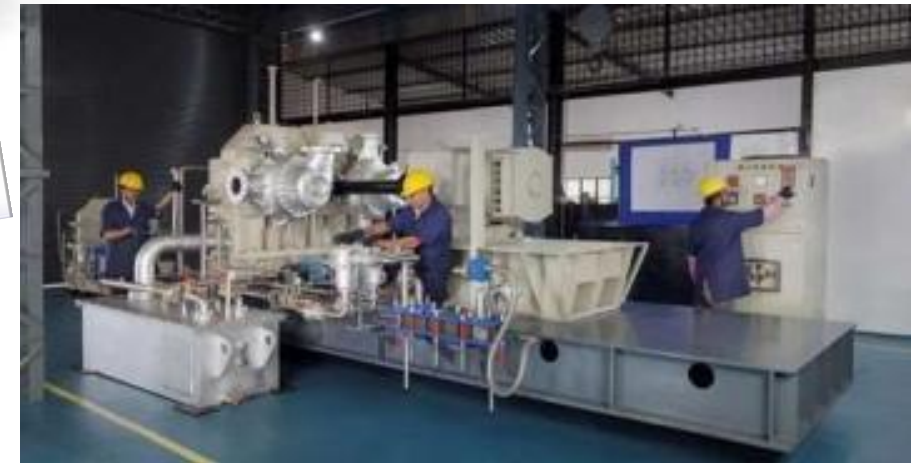
1.8 MW Condensing Turbine under Assembly
